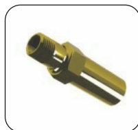
Scald Valve-dumps water exceeding 35 deg C
