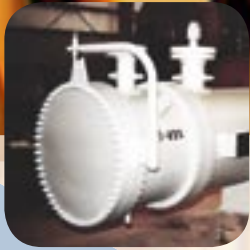
HCGO/tempered water cooler. High wall temperature achieved to limit pour-point effects. 1 shell only needed. Courtesy: Imperial Oil, Canada
