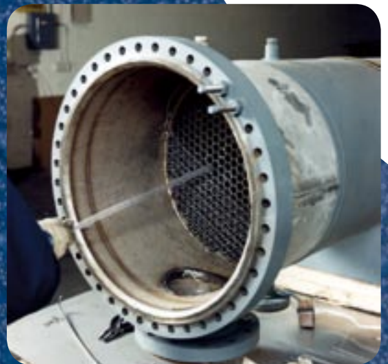
'Key Link' system being fitted to citric acid heater. Courtesy: Miles Laboratories, USA.
