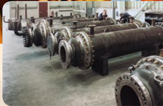
Heating crude oil with hot jacket water from pumping stations. Crude oil pipeline
