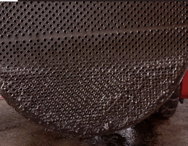
FIG. 1 A LAYER OF DEPOSIT SETTLES ON THE TUBE-SHEET
