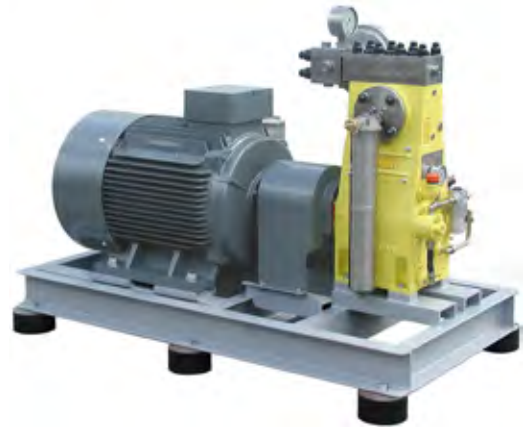
Skid-mounted - lightweight, versatile, electric or diesel options. Suitable for permanent site location.
