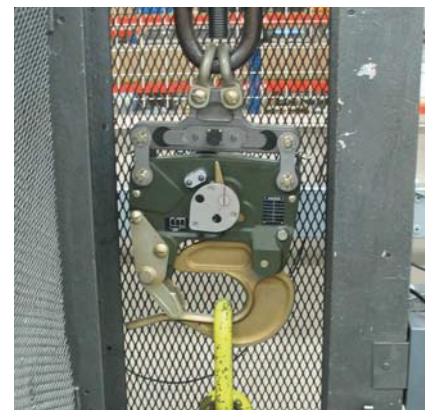
QRC and Hook being Load Tested
