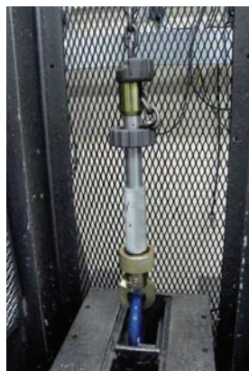
QRC and Hook being Load Tested
