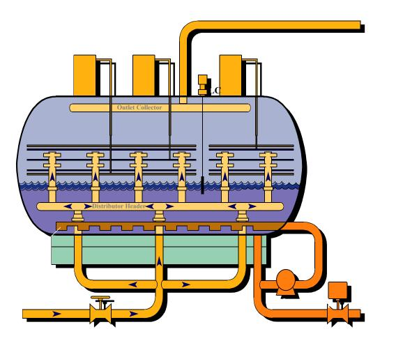
Distribution system with horizontal emulsion entry between 3 energized electrodes
